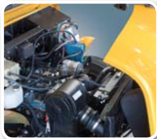
Fully integrated system, designed in complete harmony with the Engine (GM 8.1L) to ensure maximum efficiency
